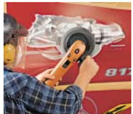
Safe sanding with dust extraction.
